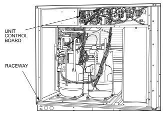
Fig. 17 — Field Control Wiring Raceway
